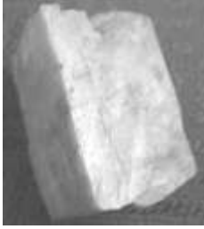
Orthoclase feldspar – 2 directions 90 degrees
