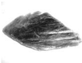
layered or 1 direction of cleavage
