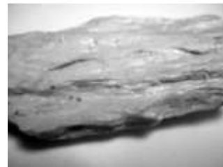
layered or 1 direction of cleavage
