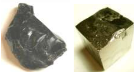
Look at broken edge of pyrite crystal for conchoidal fracture
